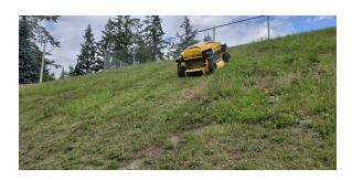
The mower also has a winch so that on the steeper slopes it can be attached to a pole at the top of the hill (you may need to have them installed if you don't have something existing) and the mower will pull itself up the hill with the winch!
